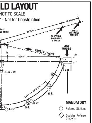
or minus six inches; target emergence elevation, high house, plus or minus three inches from level of Station 1, low house plus or minus three inches from level of Station 7. Station levels within plus or minus nine inches of Station 8 level. Mandatory referee positions should be marked.
